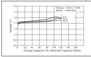
Charge temperature characteristics at various charge rates
